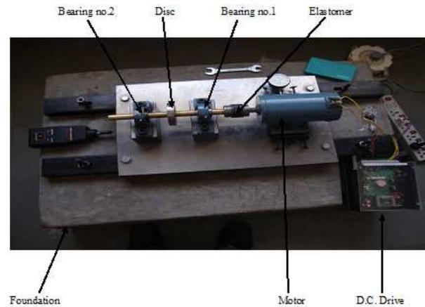
**Figure 1: Photograph of Test Rig**
